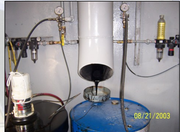
Kiln Drainage – Post Gear Shield
