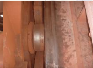
Good lube film on wear plate
