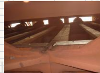
Good lube film on seal bar
