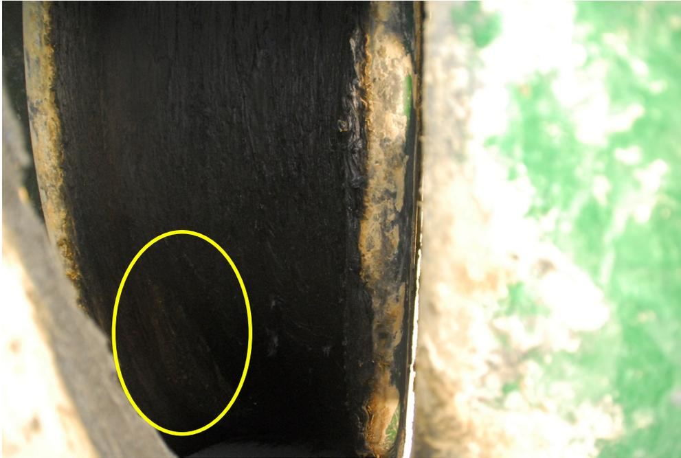
This photo of the Walking cam on the non-load side. Here you are hoping that the Walking cam lubricant adheres enough to the cam to provide some anti-rust protection.
