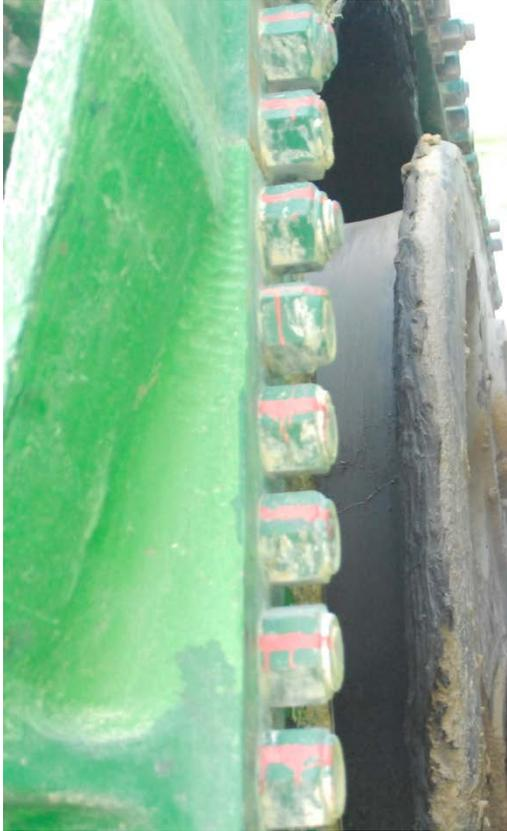
As seen in the next few photos the Walking Cam Lubricant is doing an exceptional job in protecting the cam with a heavy consistent lubricant film from edge to edge in the load zone. This dragline is 8 million pounds so each cam is lifting 4 million pounds.
