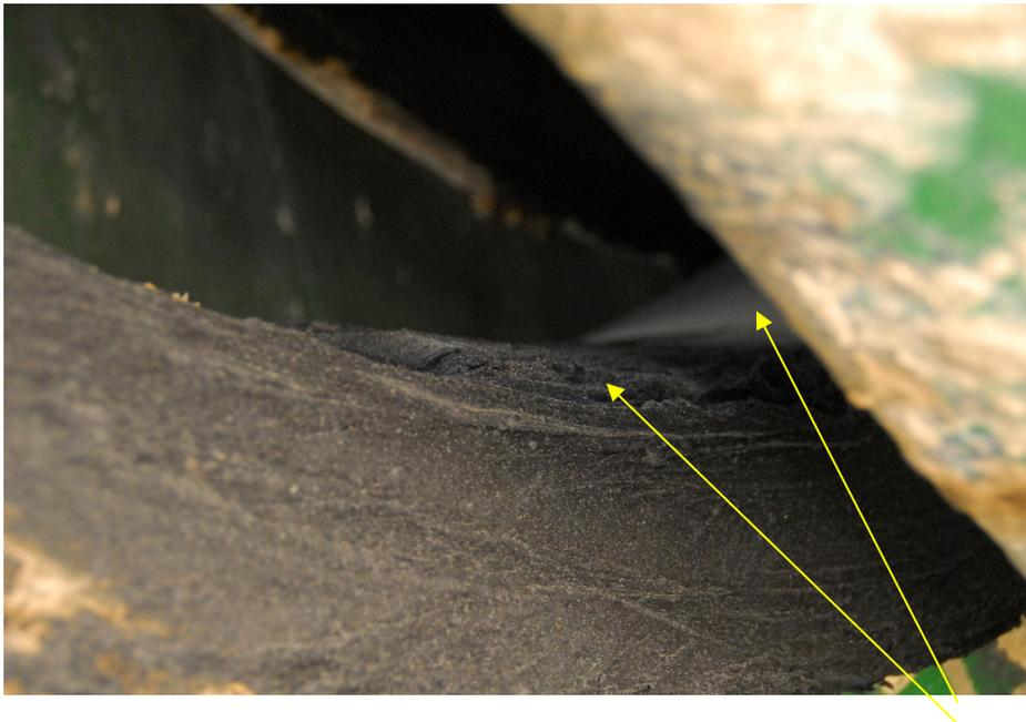
This is the transition area from loaded to unloaded. As you can see there is a grey matt appearance in the loaded area and the remainder of some previously added Walking cam lubricant has pooled up on the saddle in the non-contact zone.
