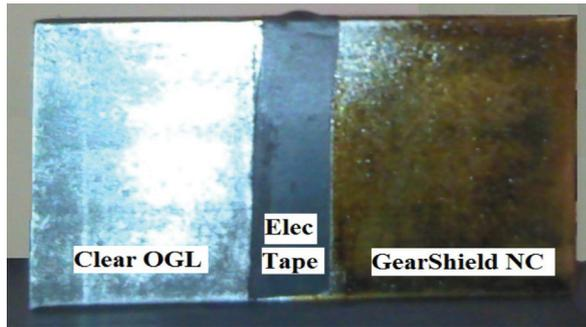
Figure 1. Test plate 0.60 emissivity (top: thermogram; bottom: photo). Clear OGL temperature: 150°F; Electrical tape temperature: 179.1°F; Gear Shield NC temperature: 173.6°F.
