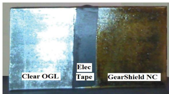
Figure 3. Test plate 0.95 emissivity (top: thermogram; bottom: photo). Clear OGL temperature: 130°F; Electrical tape temperature: 150°F; Gear Shield NC temperature: 146°F.
