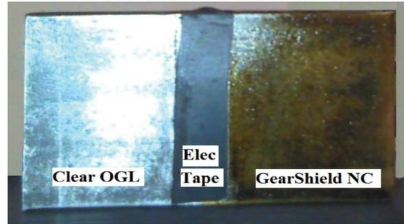
Figure 2. Test plate 0.90 emissivity (top: thermogram; bottom: photo). Clear OGL temperature: 132.4°F; Electrical tape temperature: 153.7°F; Gear Shield NC temperature: 150°F.
